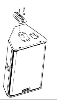
WARNING: Screws must be secured using Loctite 243<sup>™</sup>
