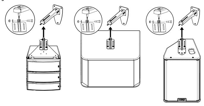
Tighten well to cancel any float between the arm and the adapter.
